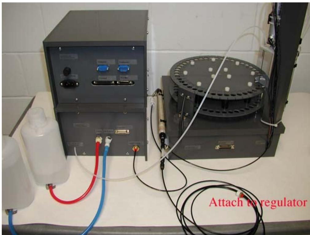
AutoMate tubing (Old version of Wet Box and Control Box shown)
